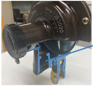
Opening (hole) to allow moisture to drain out from bonnet to prevent moisture from freezing
