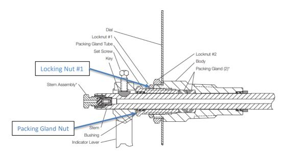
Repair kits are available for the stem & packing gland assembly.
