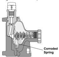
For other applications, the regulator should be inspected every 3 years.If any corrosion is evident, replace the regulator.
