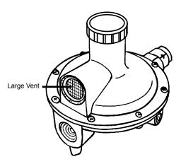
Regulators should be installed with the vent facing down or protected so their operation will not be affected by the elements. In cases where the regulator vent is equipped with a discharge tube, the outlet of this tube must be facing down. The vents and/or discharge tubes must be protected from the elements and must be equipped with a screen to prevent bugs from obstructing the opening.
