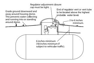
Note: Water mark left in housing dome at level above regulator vent, or end of vent tube requires replacement of regulator. Then correct installation.
