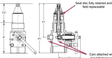
Cam attached with Allen head fastener which is accessed from the 1/4" pipe plug on side of the body
