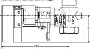
1¼" Threaded Internal Valve with Electric Actuator for Small Capacity
