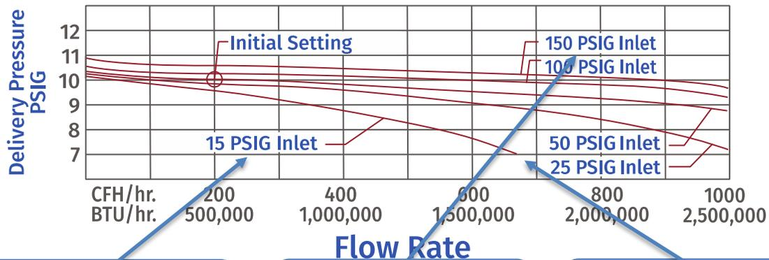
When inlet pressure goes down, delivery pressure goes down
