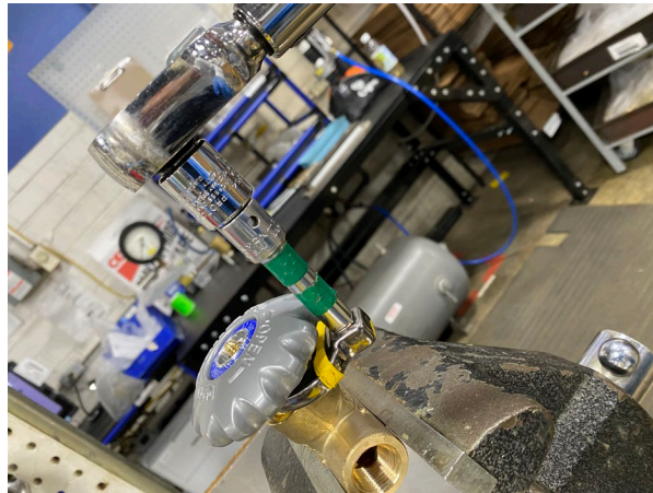
Figure 2: Final adjustment with torque wrench.
