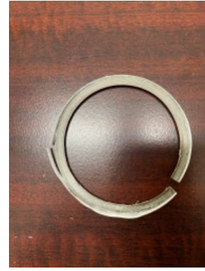
Figure 5: Over Torqued Body Gasket
