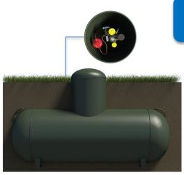
Install the regulator above the container connection and above the highest probable water level
