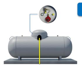
Install the regulator above the container connection underneath the lid
