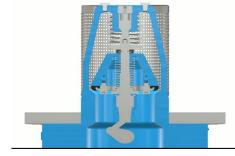
The valve opens by moving the handle to mid-point, see View "B". This position allows the actuator to put the equalizing portion of the valve stem in the pilot opening, allowing more product to bleed downstream than if the handle was fully open. In a few seconds, the tank and downstream pressure will be nearly equal. The excess flow spring will push the main poppet to the open position,
