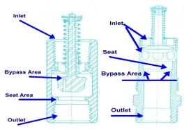
**Excess Flow Valves: Closing Flow**
